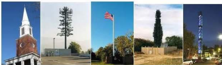
Figure 04.03-3 Examples of Concealed Facilities
