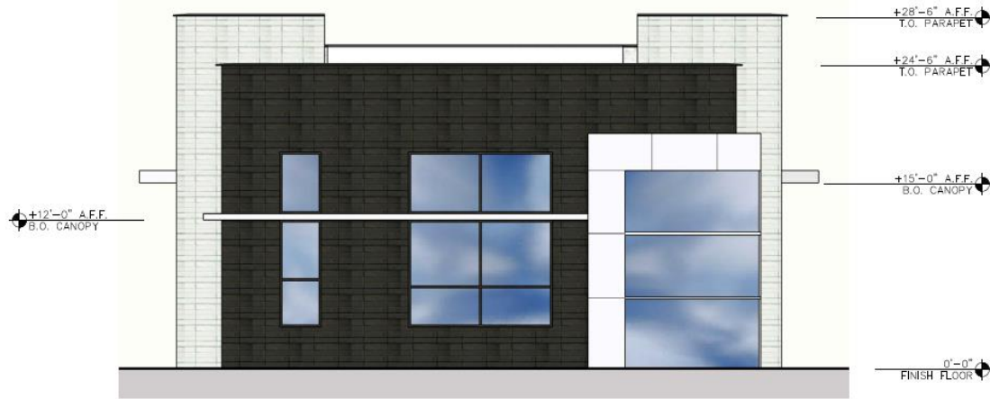
1 PROPOSED SOUTH ELEVATION SCALE: 1/8" = 1'-0"
